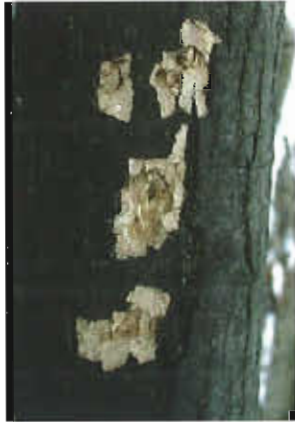
Figure 5. Jagged holes left by woodpeckers
